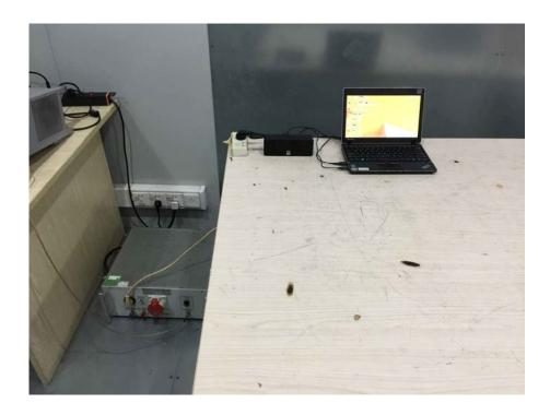
Radiation Emission Test Setup (Below 30MHz)
