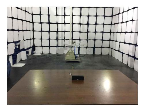
Radiation Emission Test Setup (Above 1GHz)
