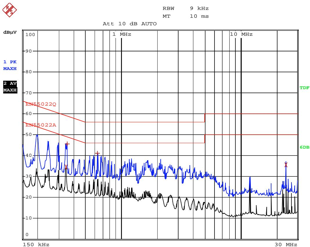
**Plot of Conducted Emissions Test Data***Conducted Disturbance**EUT: BT Drive Free 311**M/N: 1021104311-001**Operating Condition: Charging**Test Specification: L**Comment: AC 120V/60Hz USB 5V*
