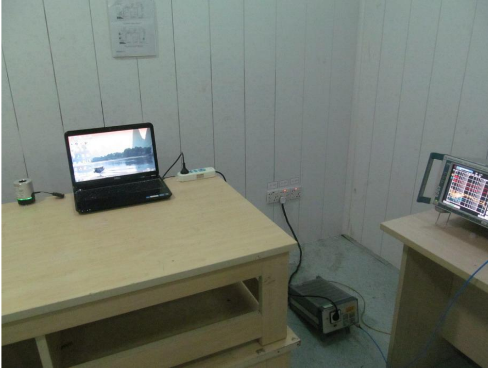
FCC LINE CONDUCTED EMISSION TEST SETUP
