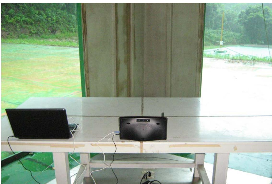
**Above 1GHz Radiated Emission Set up Photos**
