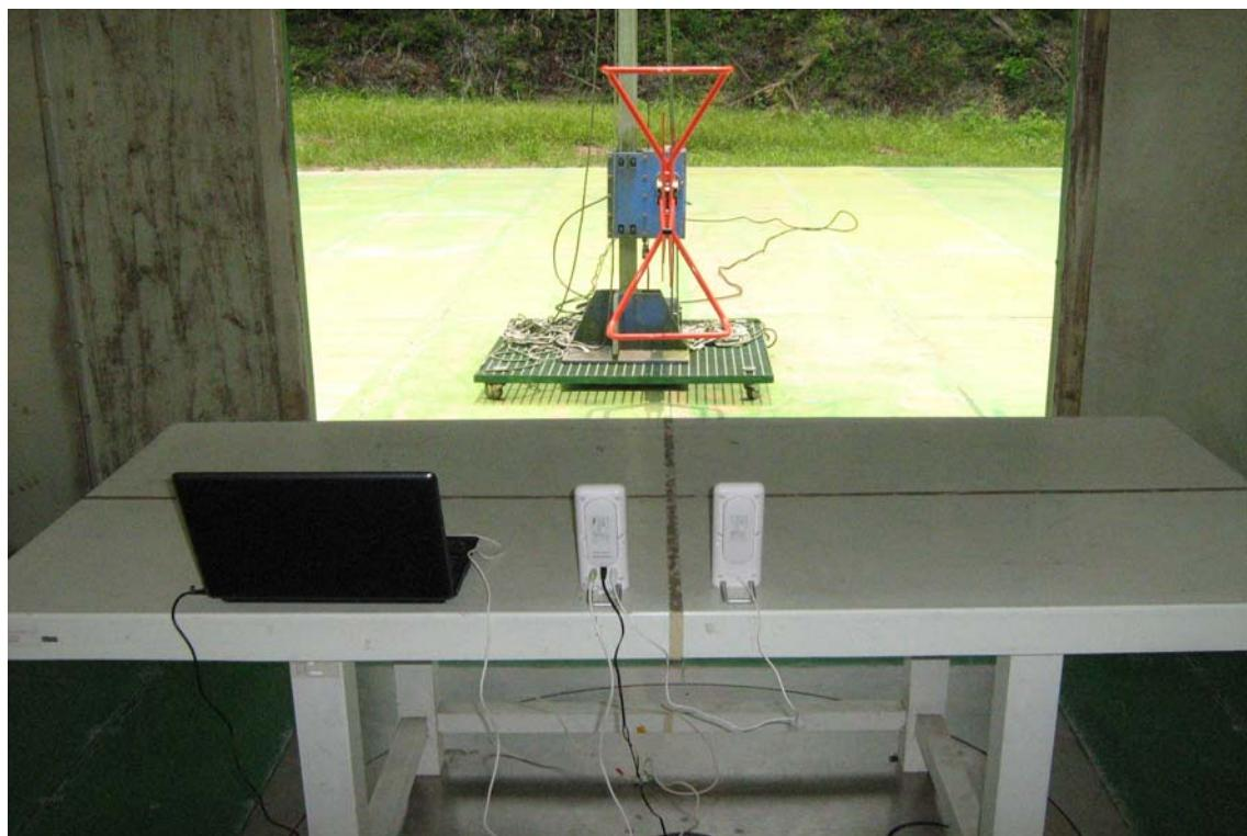
**Above 1GHz Radiated Emission Set up Photos**
