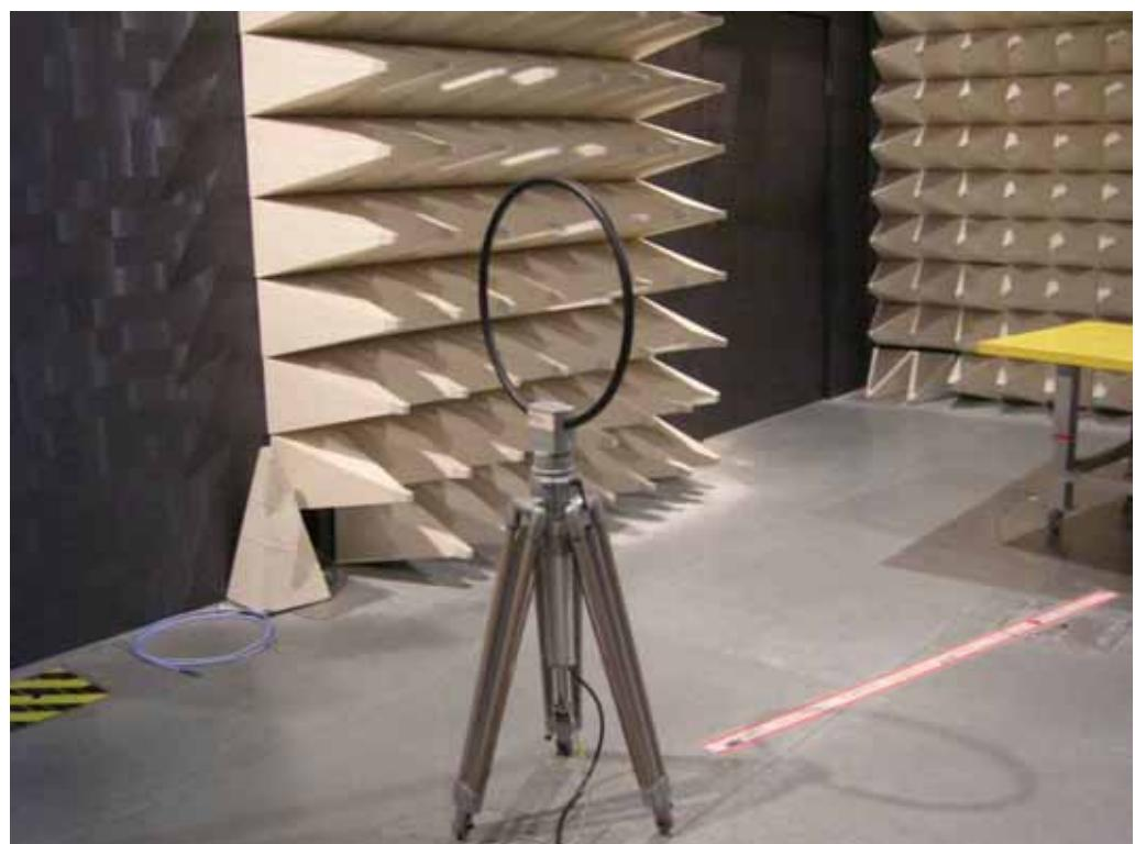
For radiated emissions 30MHz~1GHz
