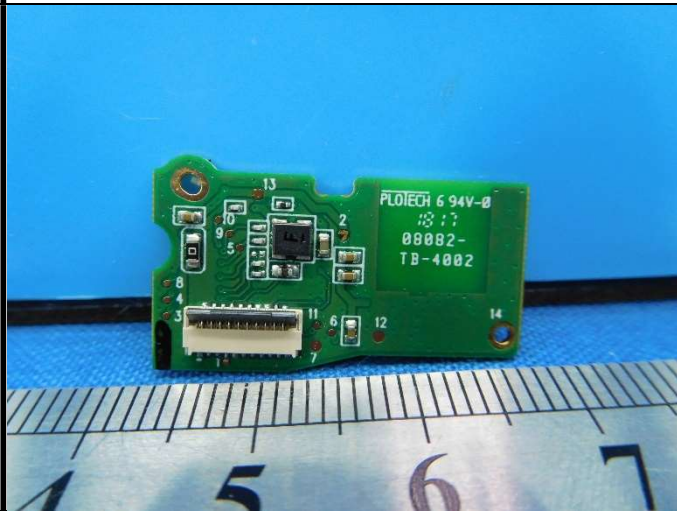
Rear Face of WLAN Module
