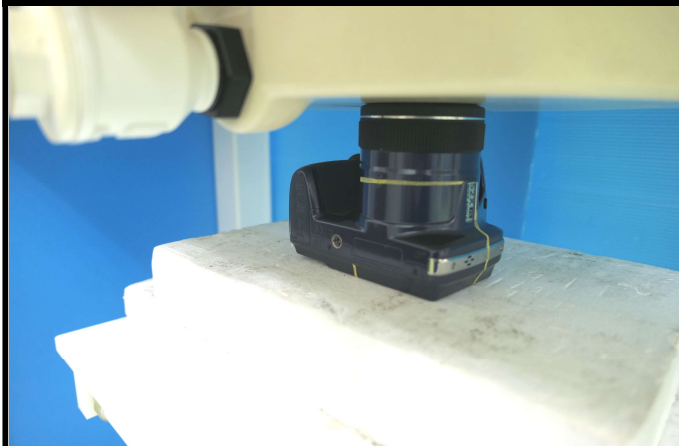
Front Face of EUT Tested at 0 mm
