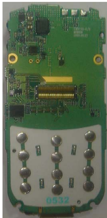
Figure 3.4 CV342/VTL601 Main Board Bottom view
