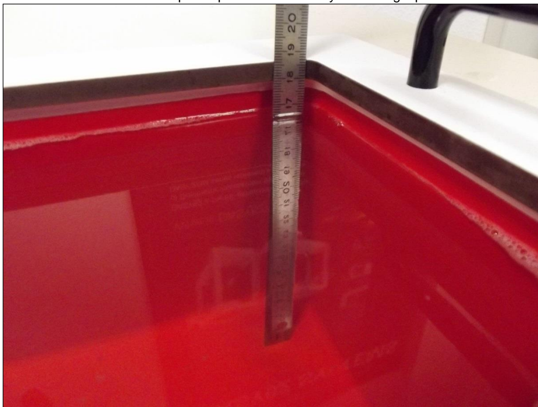
Photo 4: Liquid depth 2450 MHz body simulating liquid
