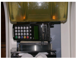
Figure 14.1 Body SAR Test Setup - Side
