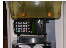
Figure 14.4 Body SAR Test Setup - Side
