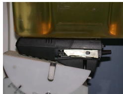
Figure 14.3 Body SAR Test Setup - Back
