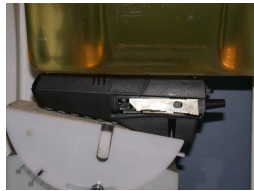
Figure 14.2 Body SAR Test Setup - Back
