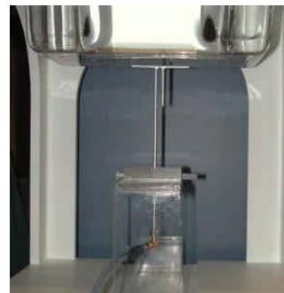
Figure 12.1 Dipole Validation Test Setup
