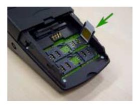
4. You can now close the slot again; the SAM will be positioned towards a plastic stop, which has the same shape as the missing corner. Gently slide the cover back to the right or left, until you hear a small click. The SAM is now firmly attached to the terminal.
