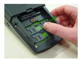
3. You can slide the SAM in the slot. Make sure the marked corner is placed correct. For the slots at the left side, the corner needs to be on your top right hand side, for the slots on the right, the corner needs to be at your down left hand side.
