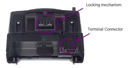
4. Install the cover on the bottom of the printer making sure that the lock and two positioning pins are clicked into the slots.
