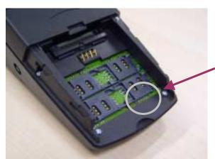
One of the four clamping mechanisms
