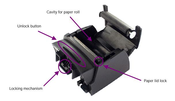
2. Position the printer horizontally at the rear side of the printer. Fit together the printer and the unit and ensure yourself that the unlock button returned to its initial position.
