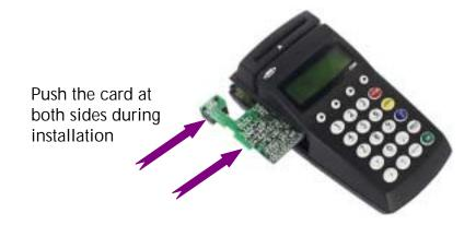
3. Slide the cover in its bottom slot and then push the upper part towards the terminal until you hear a click.
