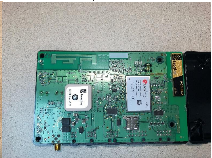
Radiated EUT top view without shield
