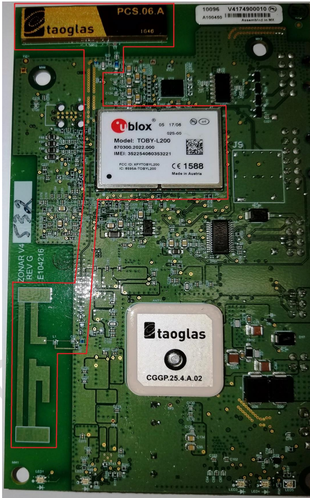
Figure 3 V4 GSM Radio Sub-Circuit
