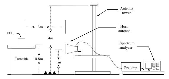
For Substituted Method Test Set-UP
