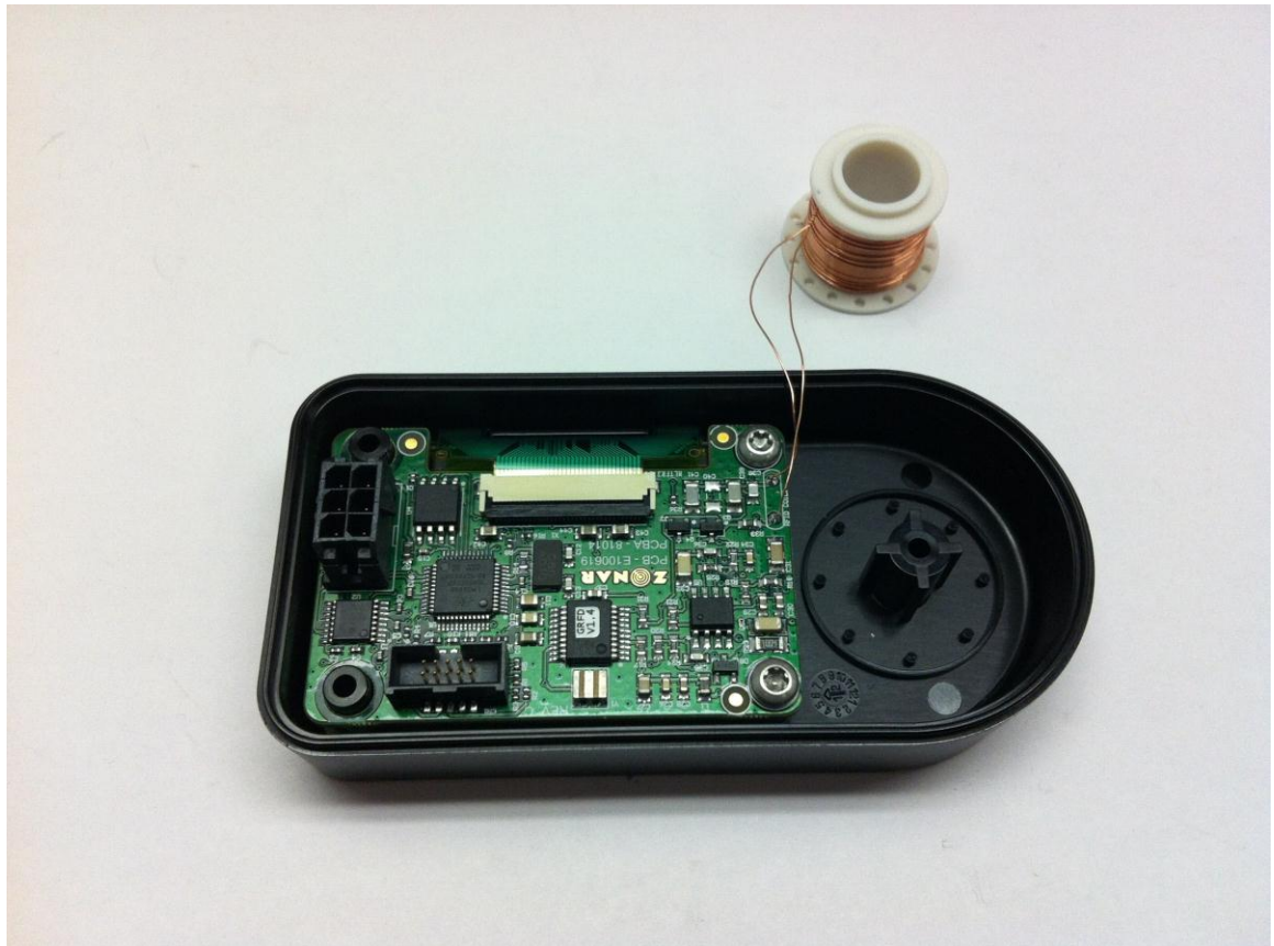
Figure 1 Coil Antenna leads soldered top right of PCB
