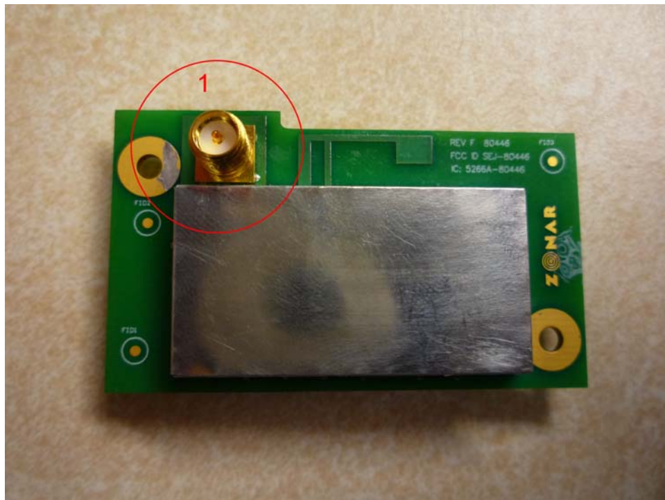
Figure 1 80446A uses a unique RP-SMA antenna connector
