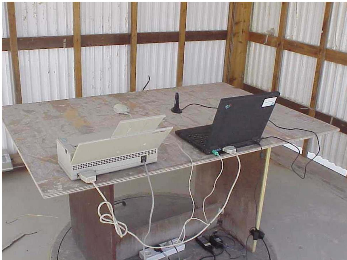
**Radiated emission test setup on Open site. Rear view**
