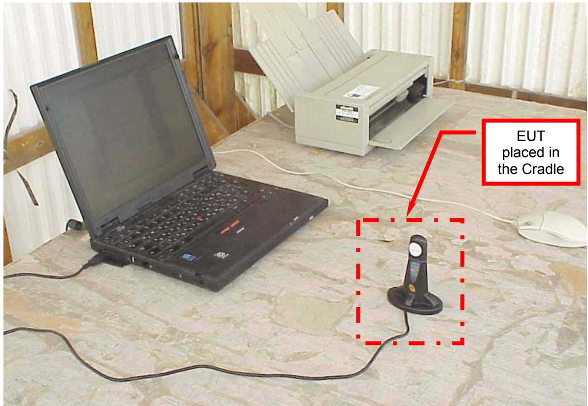
**Radiated emission test setup on Open site. Front view**
