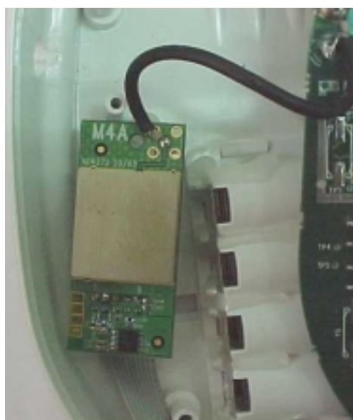
Photo 5. Tx-Rx module component side
