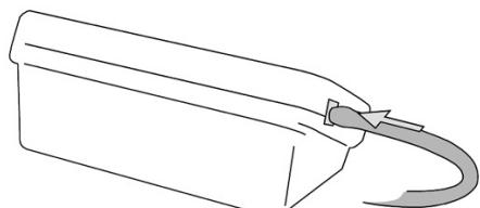
3. Wrap the cuff around the upper arm about 2-3 cm (1 inch) above the elbow, as shown below. Place the cuff directly against the skin, as clothing may cause the Wireless Blood Pressure Monitor to record a faint heartbeat and result in an error.
