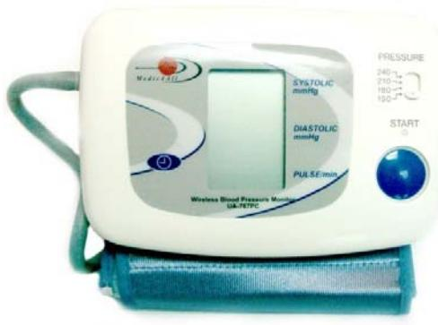
The Blood Pressure Monitor is a wireless monitoring device. It measures, stores, and transfers blood pressure and heart rate data to a medical monitoring center using the MedicGate™ or MiniGate™.
