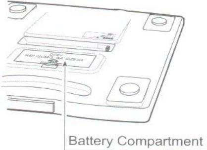
**⚠** Do not mix used and new batteries as this may cause damage to the battery or Wireless Weight Scale.
