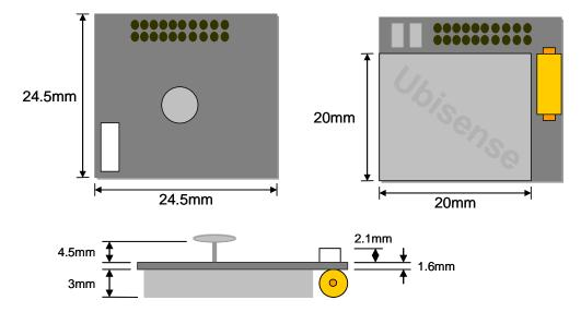
When mounting the tag on another device care must be taken to avoid occlusion of the antennas by tall components, shielding, or mounting screws. There should be an air gap of at least 1mm left around both of the antennas to avoid detuning.
