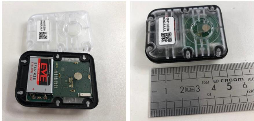
Both examples place the UBIMOD31 device inside a plastic enclosure with a battery power supply to form a location tracking tag which can be attached to objects or carried by a person – other similar integrations are possible.
