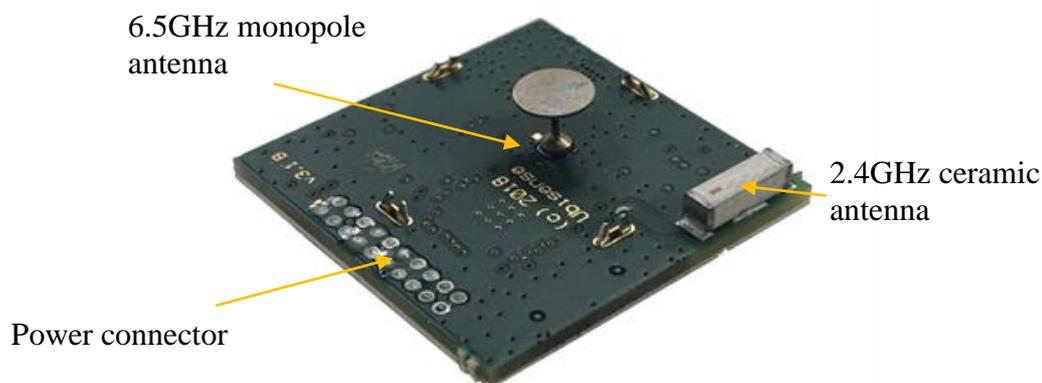
The device has two low-power transmitters – a 6.5GHz Part 15.250 transmitter which is the primary subject of our KDB enquiry, and a 2.4GHz Part 15.249 transmitter<sup>1</sup>. Note that the two transmitters are never active simultaneously.
