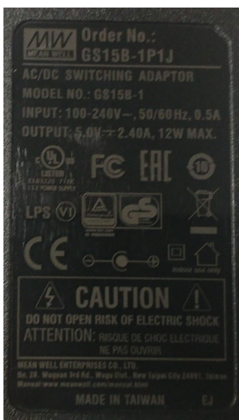
AC/DC power supply marking plate
