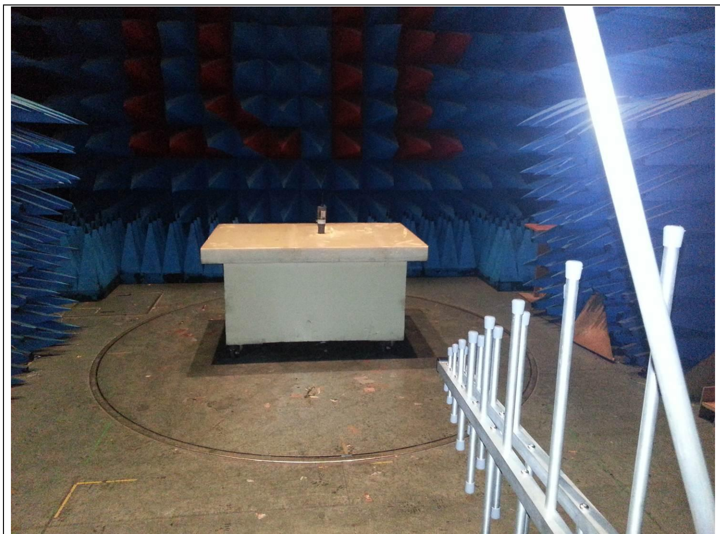
Photograph for Receiver Radiated Emissions
