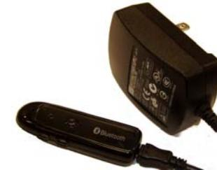
**Note:** If charging BluPAL only, you may either plug the AC/DC power converter cable directly into the base, or you may use the power y-cable, which allows you to charge both devices at the same time. When charging the Stereo Headphones you *must* use the y-cable.
