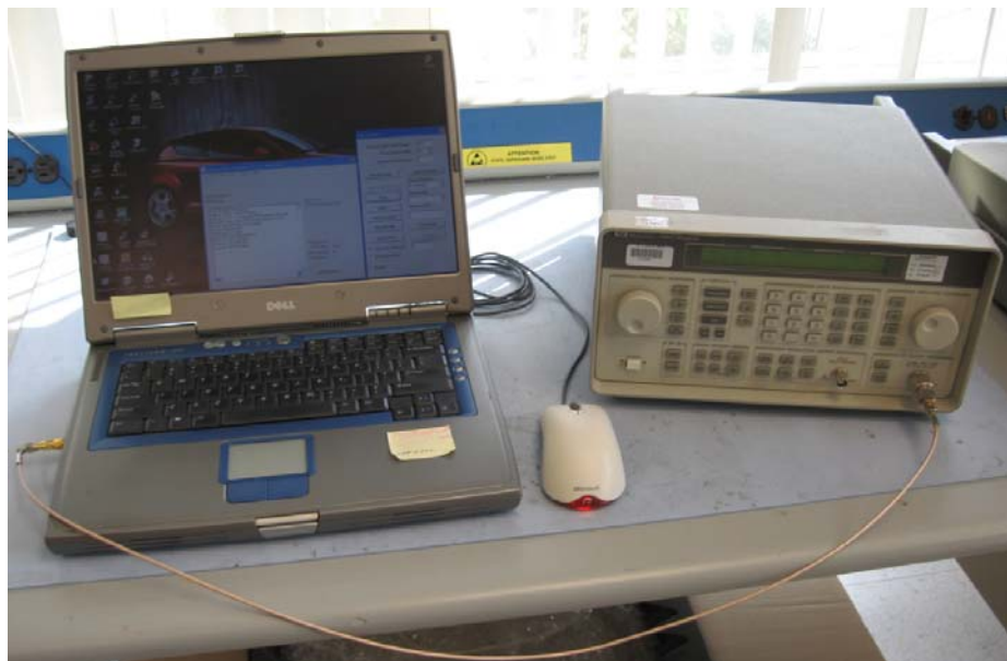
Figure 2: Test Setup for Testing the Monitoring System Threshold Power Level
