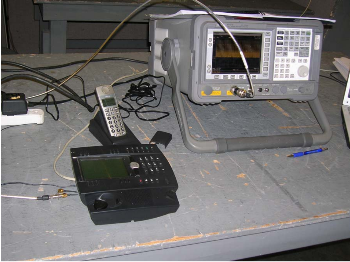
Conducted testing at the antenna port
