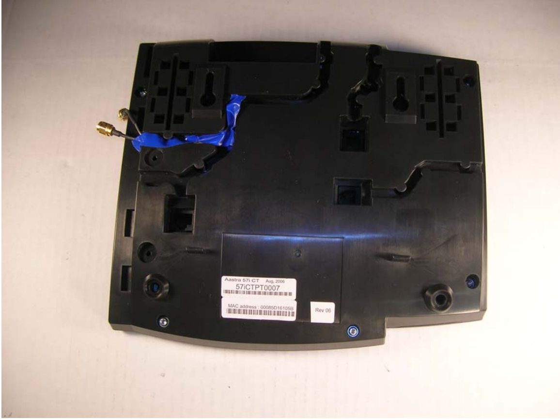
Showing dongles used for conducted testing
