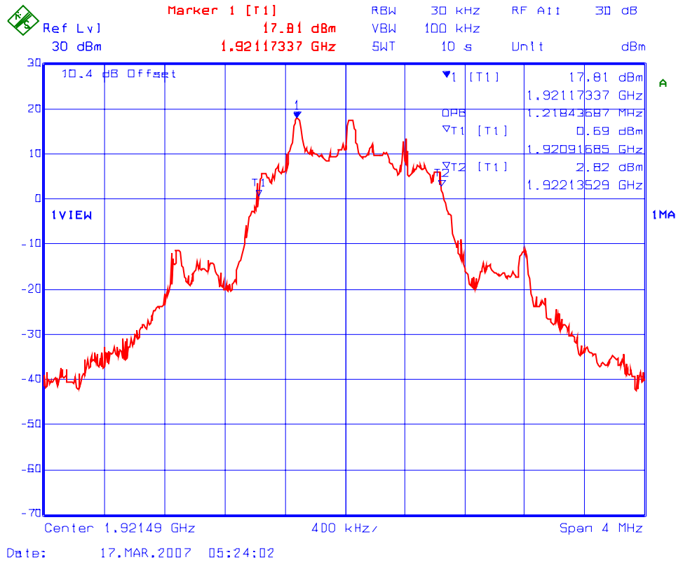
Plot 5.10.5.3 99% Occupied Bandwidth Frequency: 1921.536 MHz
