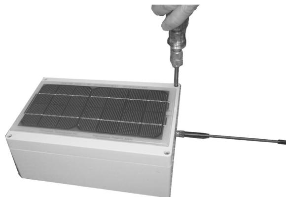
3. Lift the solar panel (lid), taking care not to damage the wiring. Disconnect the wire connectors that secure the wiring between the solar panel (lid) and the charging circuit board (in the chassis). Rest the lid on the ground.
