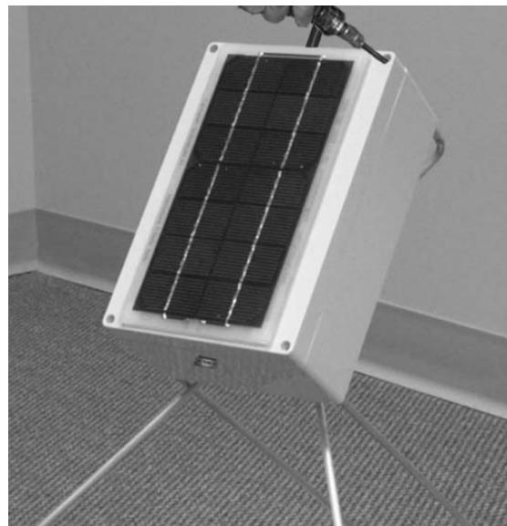
3. Temporarily secure the base of the legs to the roof. Leave the unit for a day, so it is exposed to a cycle of sunlight and darkness.
