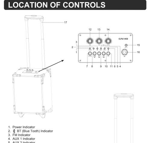
Power Indicator 2. \* BT (Blue Tooth) Indicator AUX 1 Indicator 5. AUX 2 Indicator 6. 🗷 Charging Indicator 7. SOURCE Button 8. SCAN / ►II (Radio Scan/Play-Pause) Button 9. CH - / I◀◀ (Channel Down/Skip Backward) Button 10. CH + / ▶▶I (Channel Up/Skip Forward) Button
