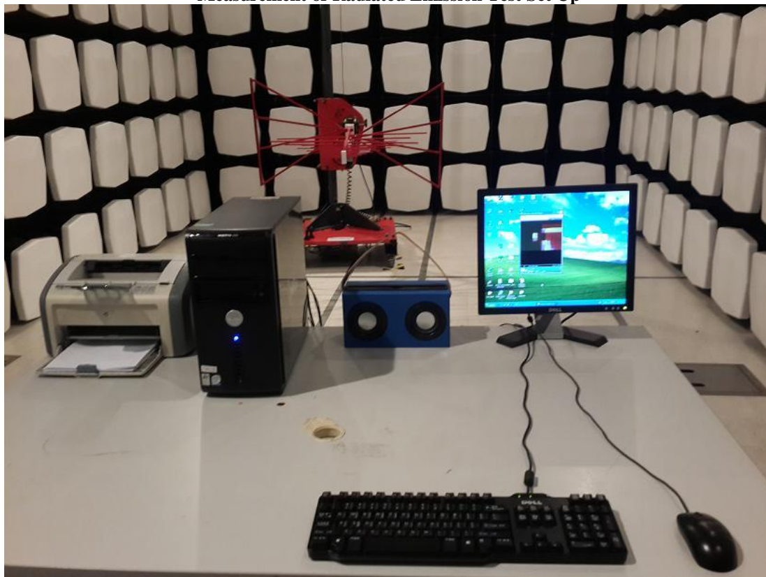
Measurement of Radiated Emission Test Set Up
