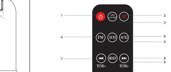
7. TUNE -/I◀◀ (Skip Backward) Button 8. TUNE+/▶►I(Skip Forward) Button RESET Button When there is an obstacle between the unit and the transmitter, the transmitter may not operate. 11. VOL (Volume) - Button When direct sunlight, an incandescent lamp, 12. VOL (Volume) + Button fluorescent lamp or any other strong light shines
