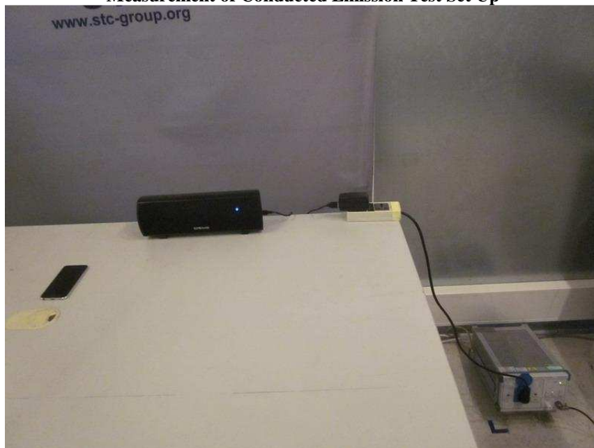
Measurement of Conducted Emission Test Set Up
