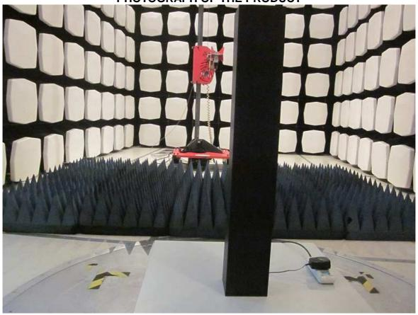
MEASUREMENT OF CONDUCTED EMISSION TEST SET UP
