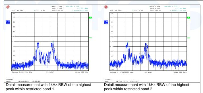
Output power (conducted): -71.0 dBm/kHz
