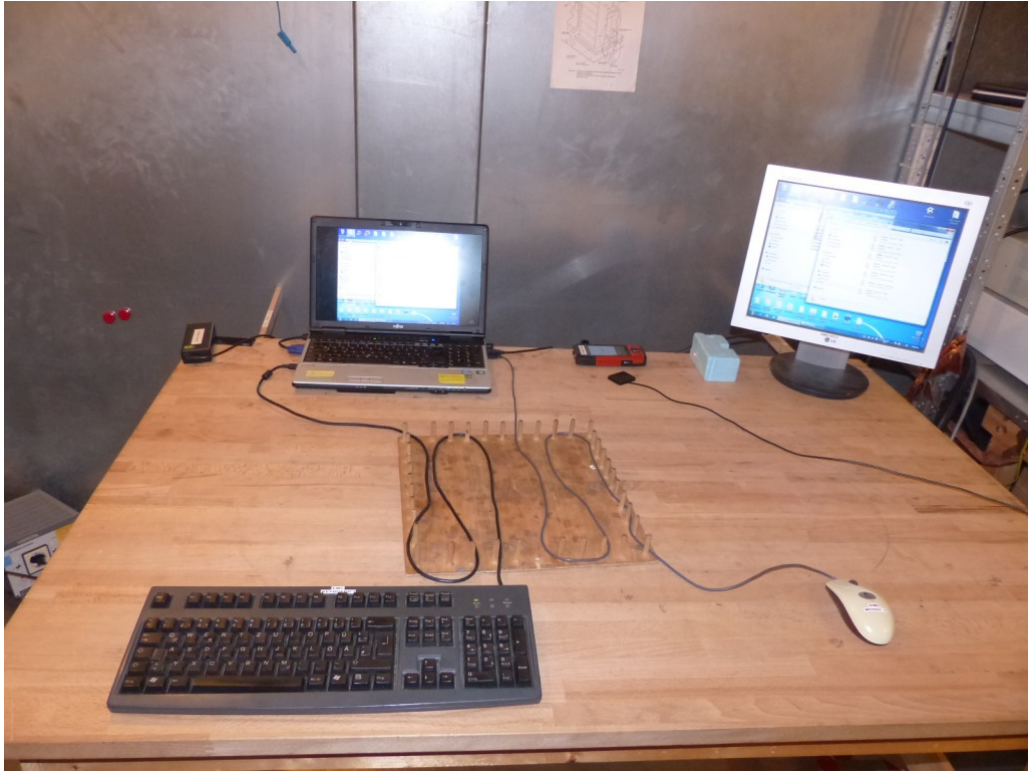
Photo 5: Test setup for conducted measurements (computer peripheral setup, EUT supplied by USB-cable from computer, charging mode, unintentional radiator §15)
