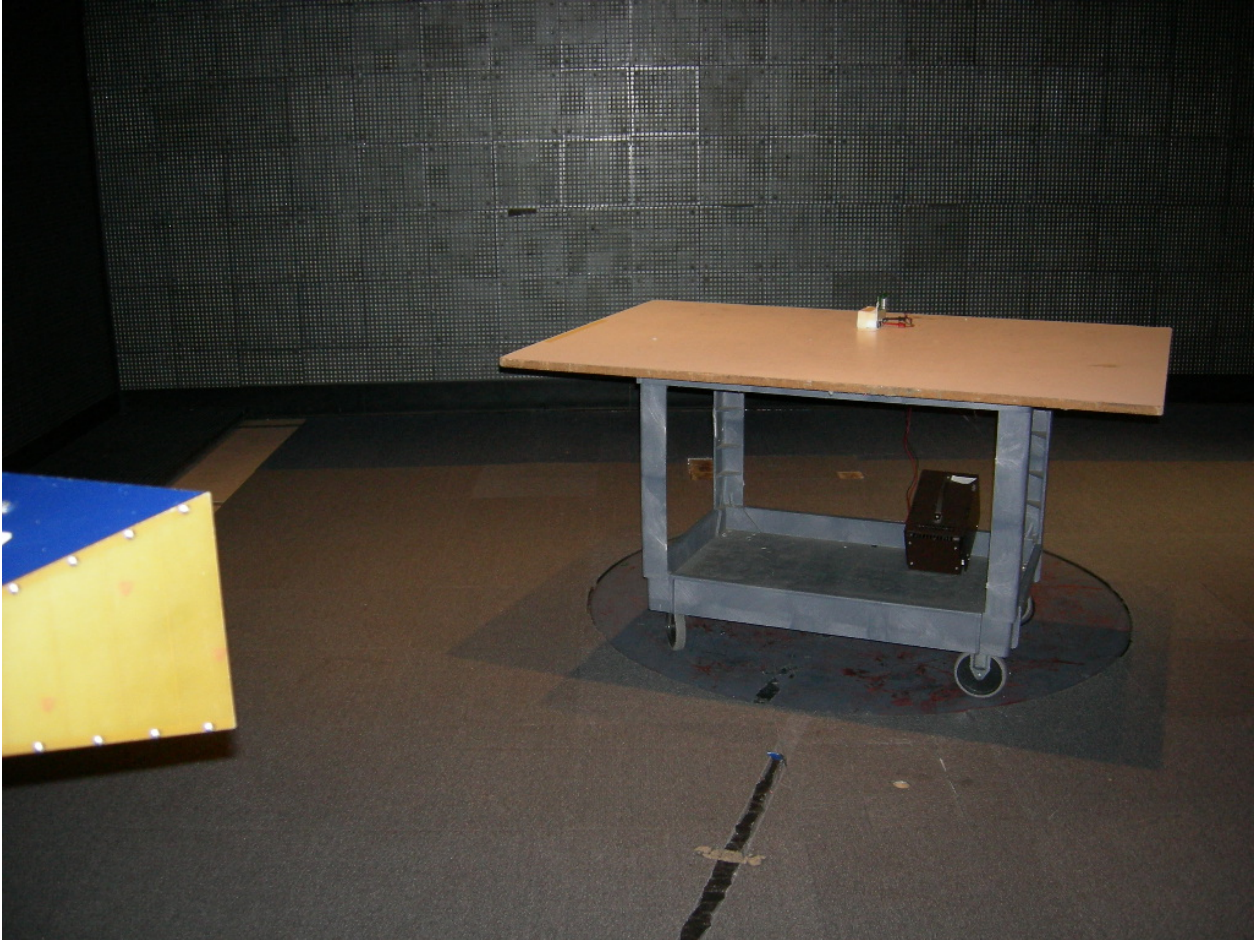
Figure 5: Radiated Emissions (510x SOH Board)
