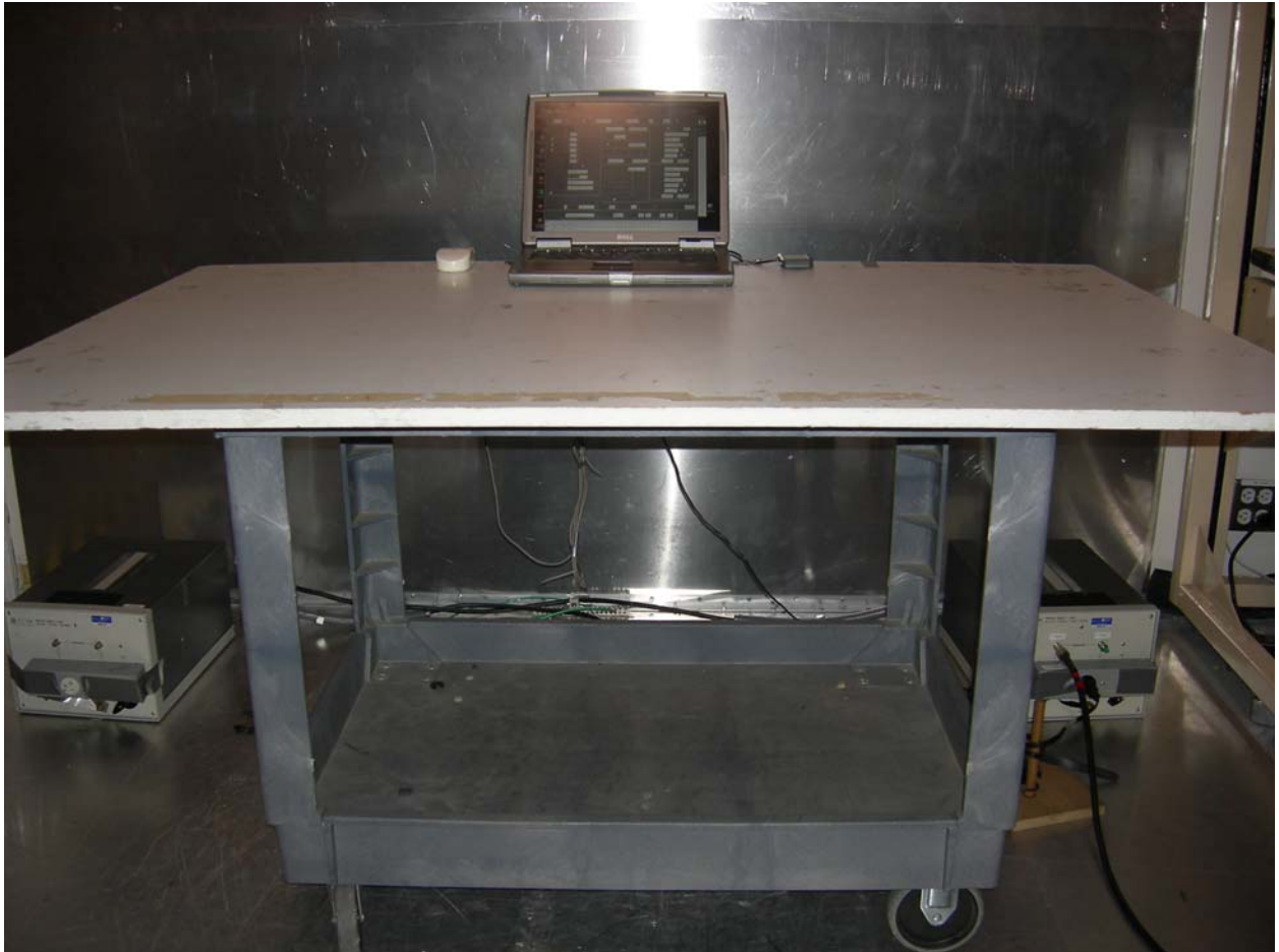
Figure 4: AC Power Line Conducted Emissions
