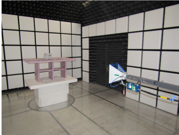
Figure 1: Radiated Emissions – Front – Above 1GHz
