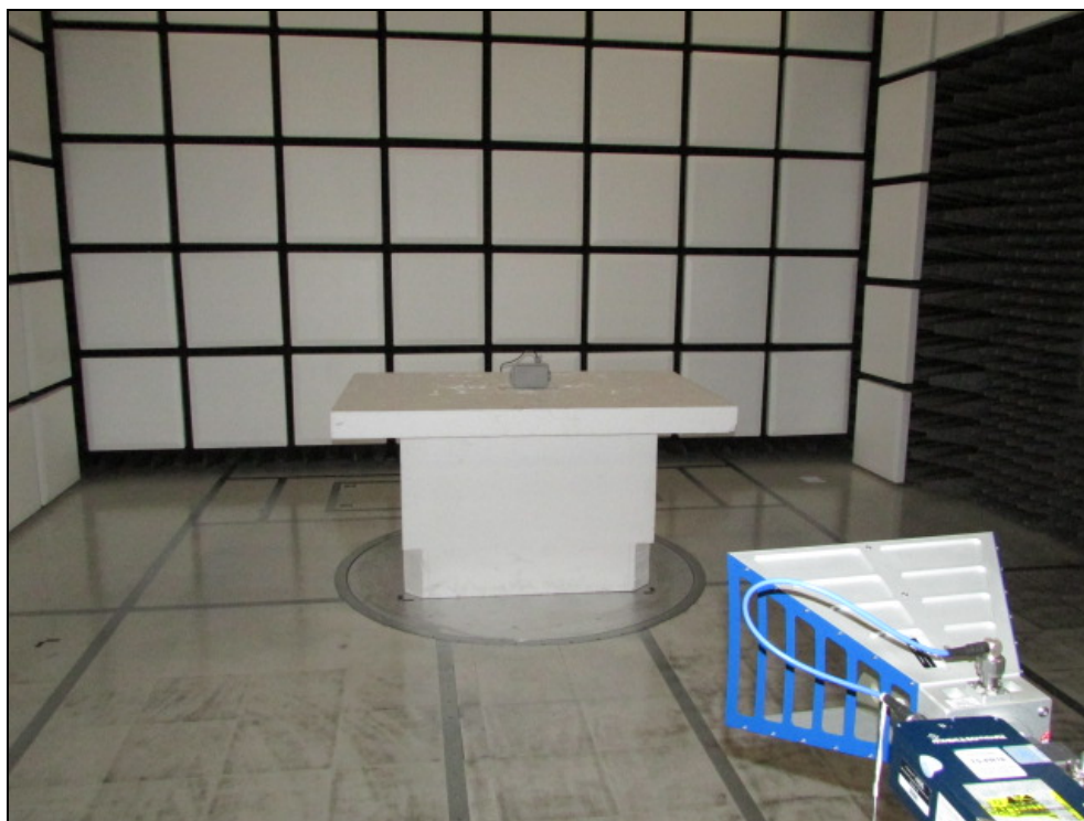
Figure 3: Radiated Emissions – Front View – Above 1GHz
