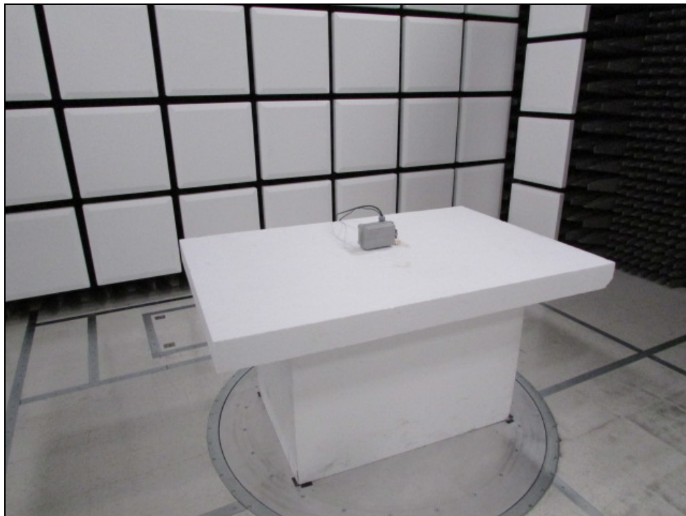
Figure 1: Radiated Emissions – Front View – Below 1GHz
