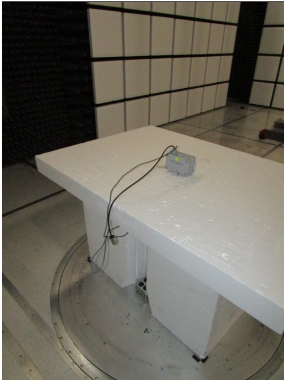
Figure 2: Radiated Emissions – Rear View – Below 1GHz
