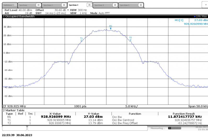
Figure 2.3.6-18 - 99% Bandwidth – KDS TCXO – 928.925 MHz - 2FSK Mode
