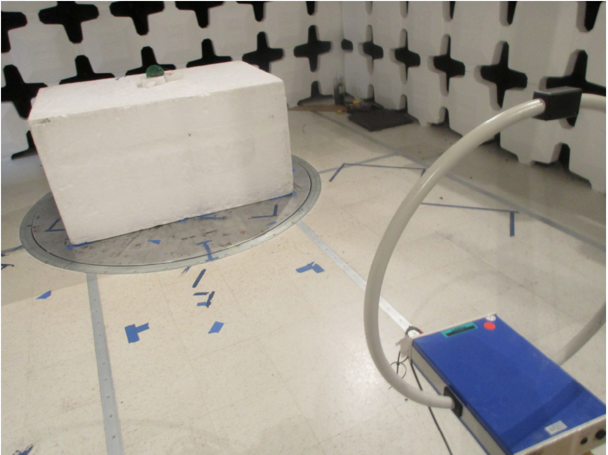
Figure 1: Radiated Emissions – Front View – below 30 MHz
