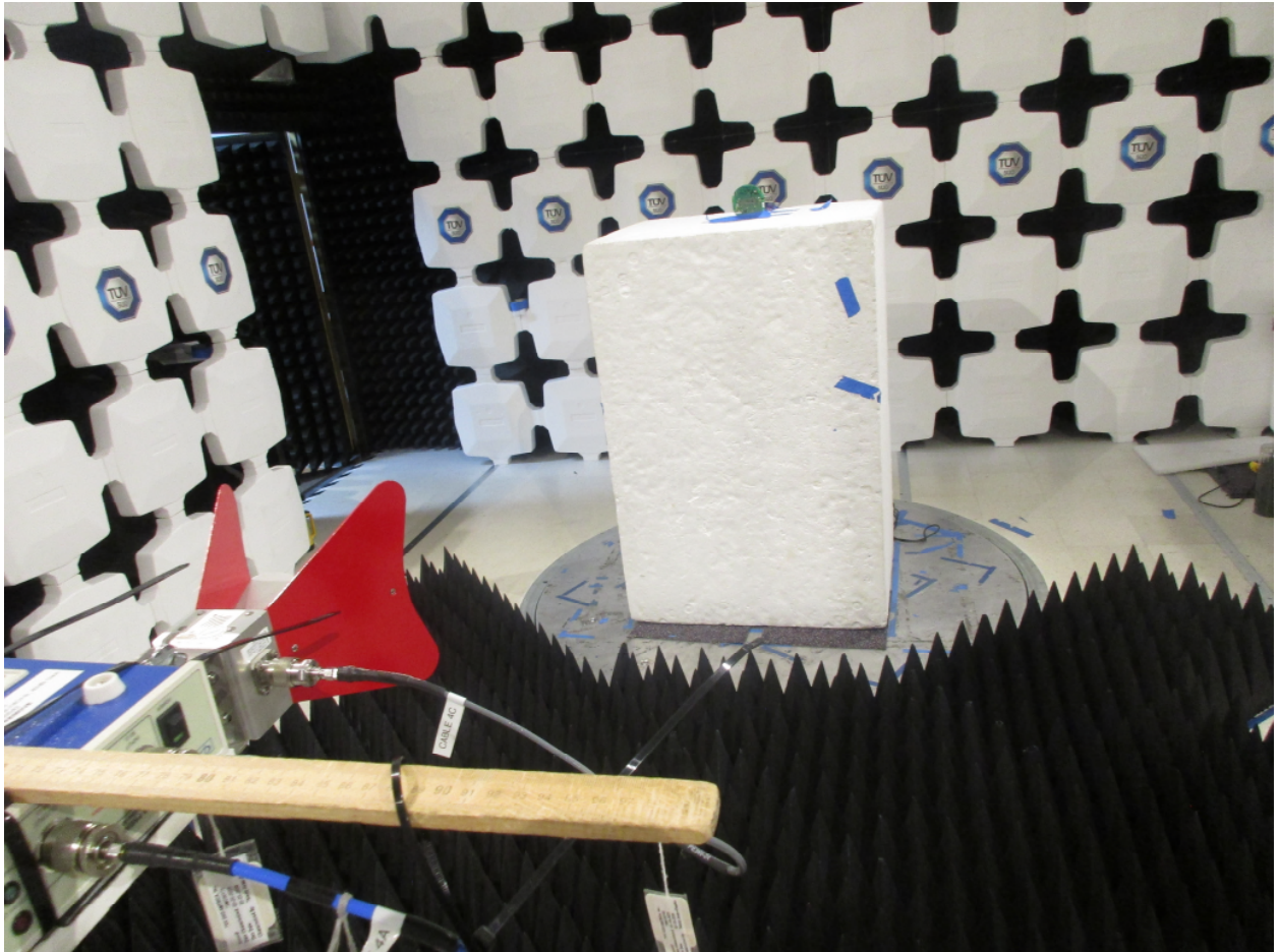
Figure 5: Radiated Emissions – Front View – above 1 GHz
