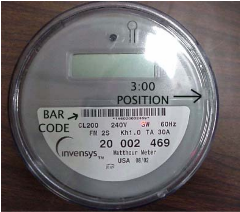
Photograph showing bar code position and 3:00 position for programming wand placement on meter.
