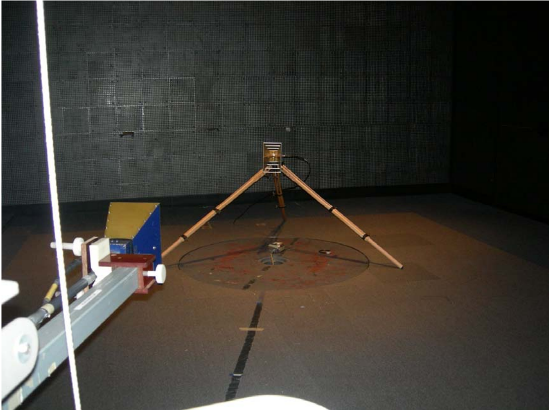
Figure 3: Radiated Emissions – Substitution
