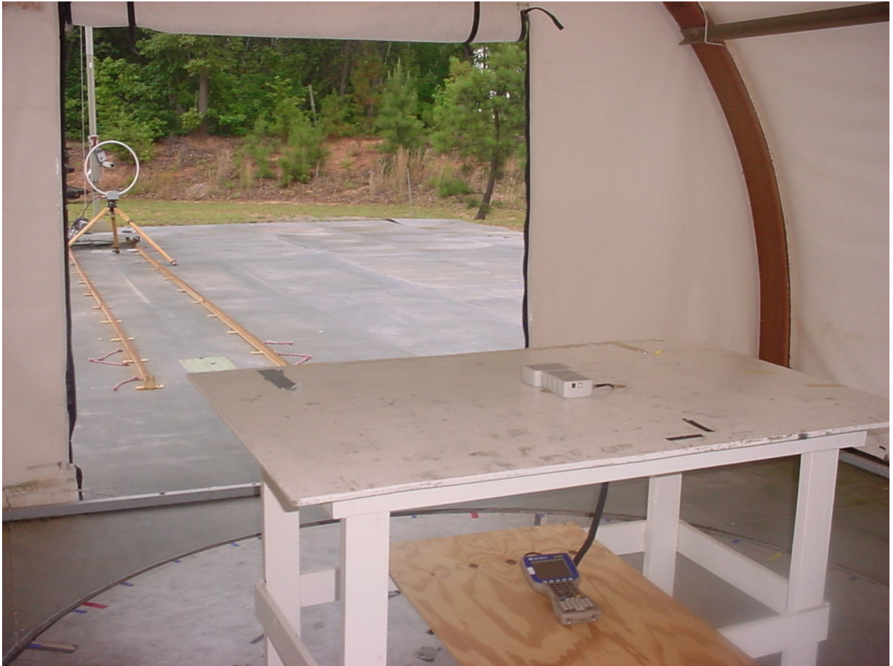
Figure 1: Test Setup – Radiated Emissions < 30MHz
