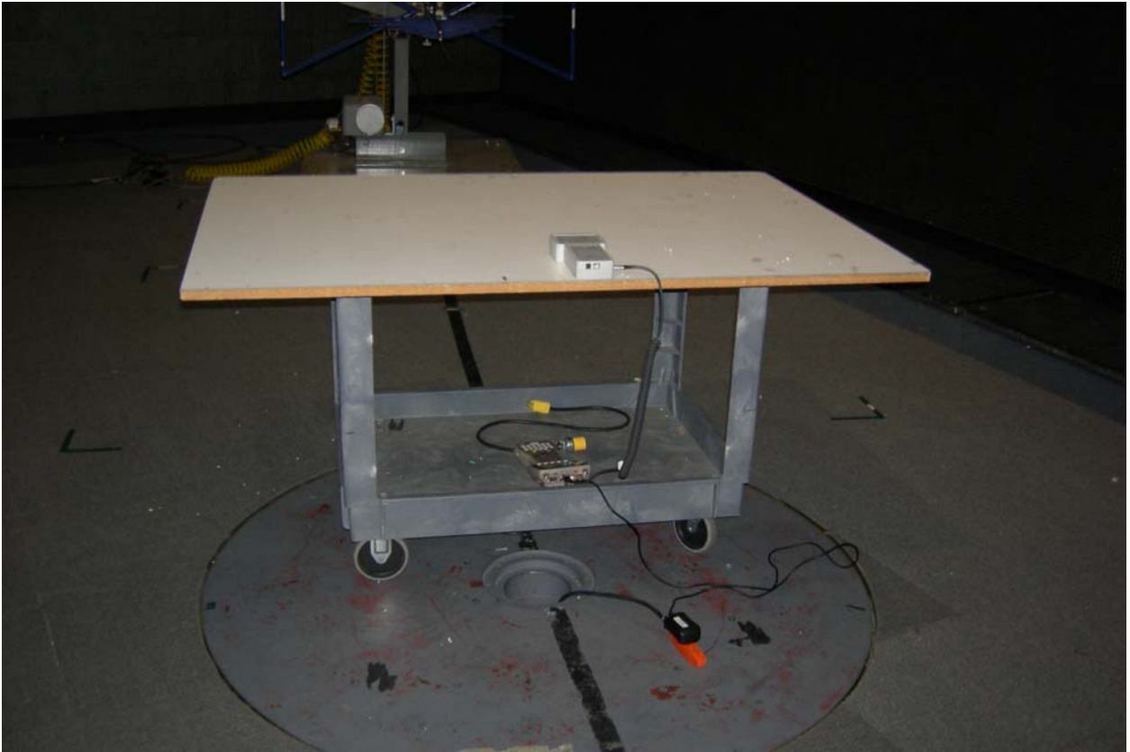
Figure 2: Test Setup – Radiated Emissions > 30MHz
