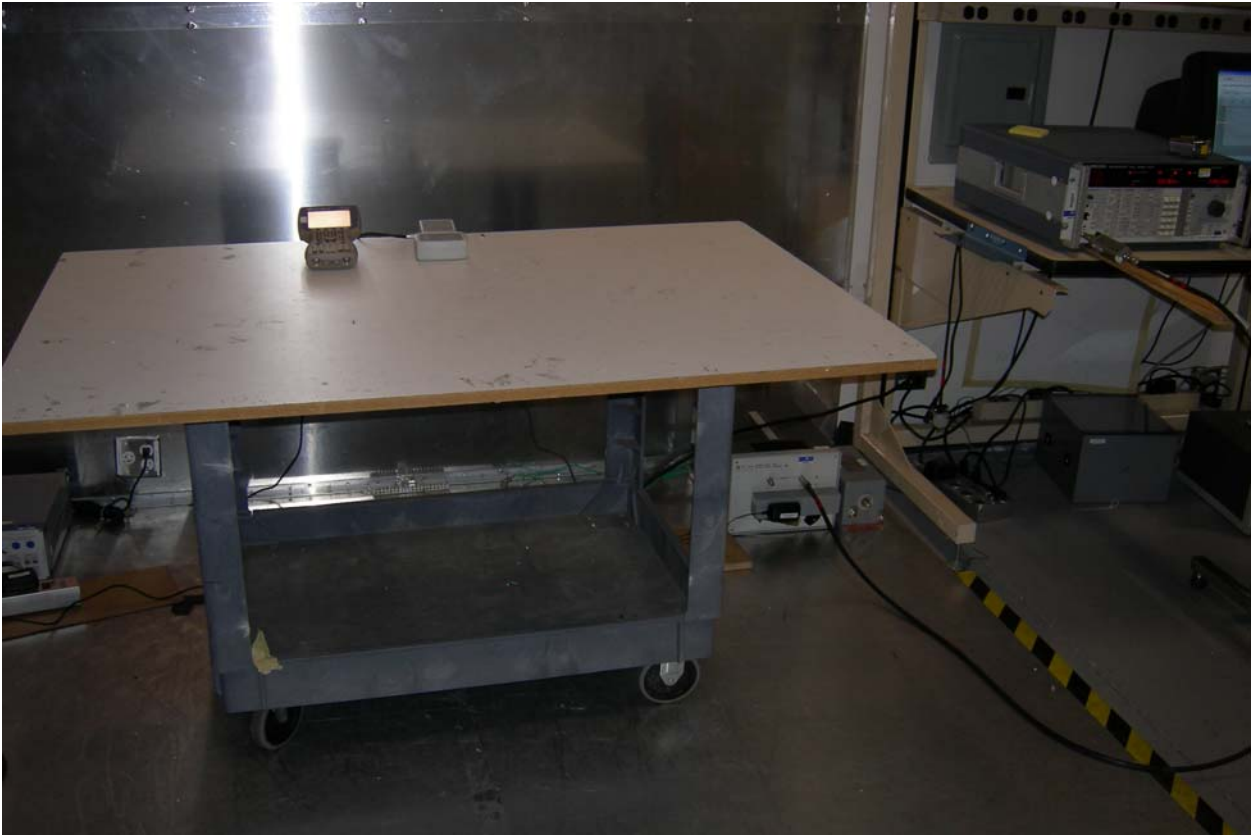
Figure 3: Test Setup – AC Power Line Conducted Emissions
