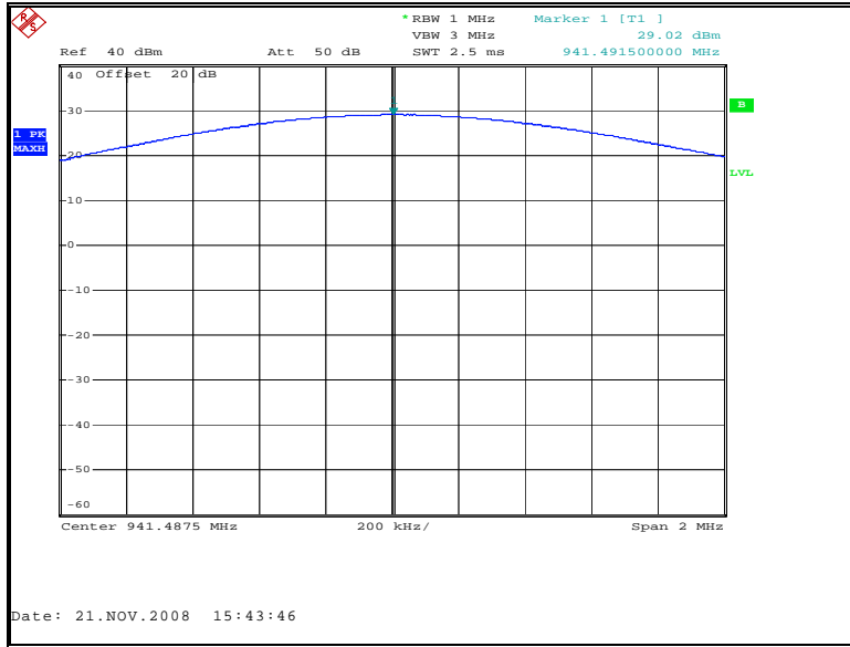
Figure 7.1.2-7: Peak Output Power 941.4875 MHz
