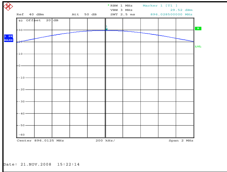
Figure 7.1.2-3: Peak Output Power 896.0125 MHz
