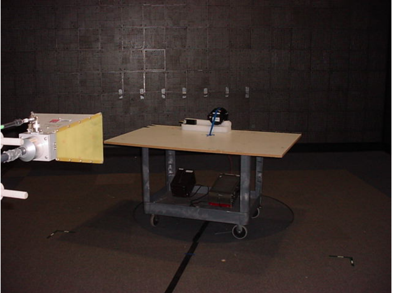
Figure 2: Radiated Emissions – Transmitter Front View
